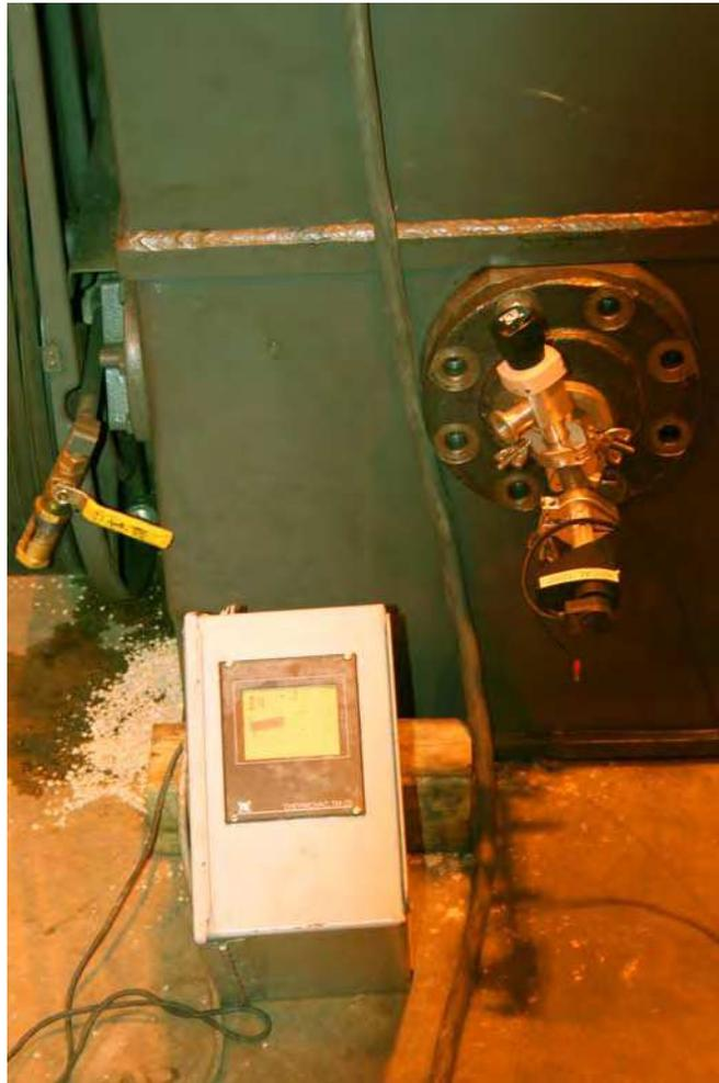
If you suspect there's a problem with your pumping system, isolate the pump from the chamber and run a "blank-off test" to evaluate it. You can close the roughing valve and test the ultimate pump pressure with a Pirani gage when it's included with your system. Otherwise, use a blank-off plate on the pump's inlet (see photo). This pump is "basing" at  $3.4 \times 10^{-1}$  Torr or 340 microns. It has a bad shaft seal, causing a high base pressure.
