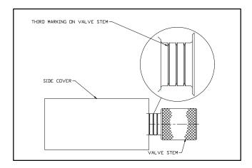
3.4.1 Open the Gas Ballast valve for maximum efficiency. For a lesser degree of ballasting, turn valve toward close position. Full gas ballast will cause pump temperature to rise but this is normal. For maximum effect of gas ballast, pump should be run at approximately 160 Deg. F. (71 Deg. C) Operating temperature can be raised by throttling cooling water. Oil temperature control kits are available from the factory. Consult Stokes Vacuum for specifications.
