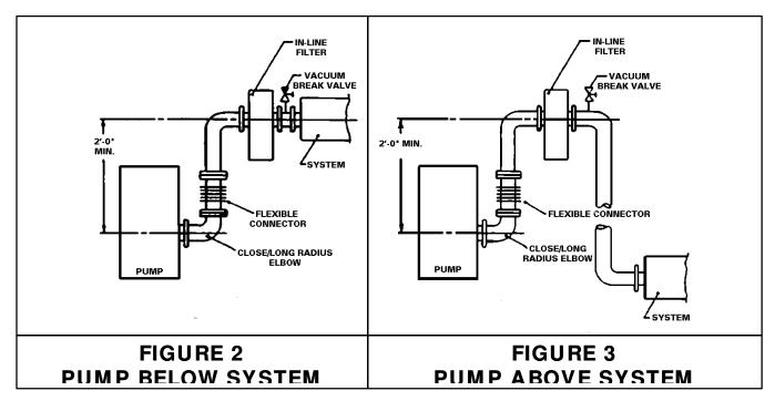
A high vacuum valve (full opening type preferred) is recommended to facilitate start-up and for checking pump blank off pressure.
