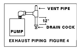
2.3.1 It is recommended that the exhaust be piped horizontally a short distance and tied into a vertical exhaust pipe. The vertical exhaust pipe must be at least 12" (305 mm) long with the bottom end terminated with a plug or a drain cock to allow removal of moisture and contaminated oil before it can accumulate sufficiently to drain back into the pump oil reservoir. See Figure 4.
